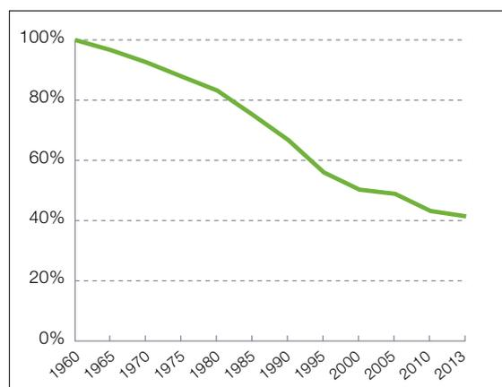
Figure 1: Indexed global energy consumption/tonne of crude steel production
